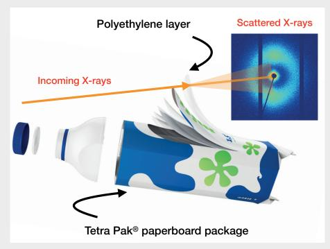
Polyethylene layers act as a barrier and adhesive for Tetra Pak® paperboard packages. X-ray scattering measurements on one of the polymer films show that crystals in some films have a preferential orientation originating from the process used to produce them. What we did
