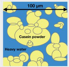
The measured SESANS signal (left) changed with time as the large, irregularly shaped casein powder particles (right) were rehydrated by heavy water ( $D_2O$ ). The change in the signal is related to the amount that the powders had been rehydrated.
