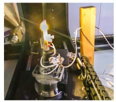
In situ measurement setup showing the running LED "sandwich" within the X-ray CT equipment.
