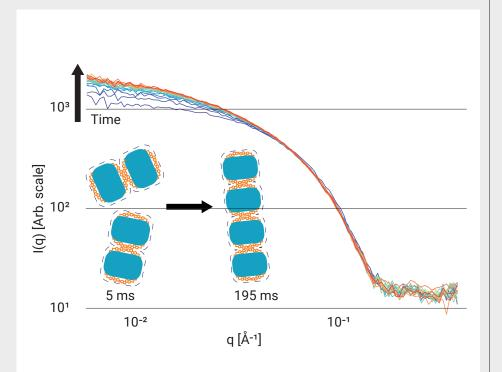
When insulin is transferred to a water based solvent that mimics the conditions when injected, it undergoes a structural change. This change is observed on a millisecond time-scale with the stopped-flow SAXS technique.
