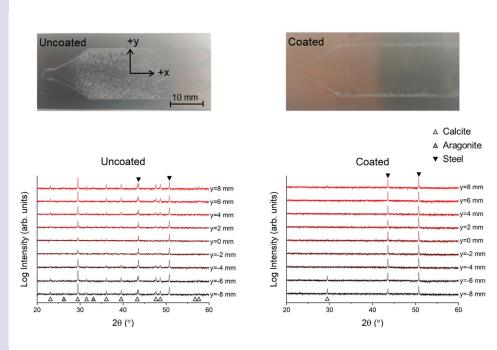
Upper: Selected steel surfaces after 40 hours exposure in an accelerated heat exchanger environment. Lower: Corresponding X-ray diffraction patterns collected at a fixed x position in steps along y
