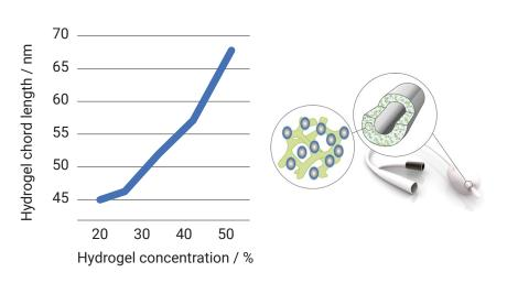
Soaking Biomodics IPNs in heavy water ( $D_2O$ ) highlights the hydrogel structure when analysed with neutrons. This enables a determination of characteristic sizes from the SANS data. One important parameter is the chord length, which is a measure of the average size of the hydrogel domains.
